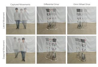
Figure 3: Comparison of omnidirectional drive and differential drive controls in replaying lateral and diagonal movements. Note that differential drive was simulated using omnidirectional wheels by adding similar constraints.
