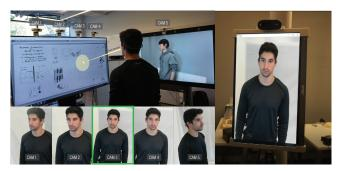
Figure 4: We used multiple servo-controlled cameras in our initial approach for rendering a front face, but then discarded them in our final design.
