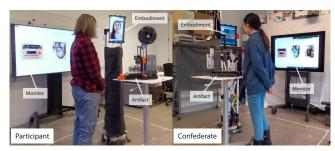
Figure 8: The ReMotion setup used for our user study showing the two symmetrical settings. There is a table used to place the artifact and a display monitor used to present three aspects of the artifact.
