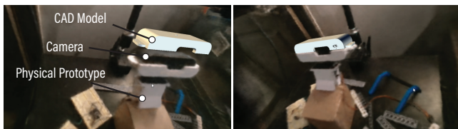
Figure 17: A CAD model can be rendered with actual dimensions in NeRF rendering and moved over the physical prototype to ensure that it fits well with the camera before it takes a long time to 3D print it.
