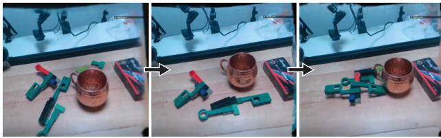
Figure 6: NeRF scene updates after each detected alternation in the task space. The last two snapshots were taken seven seconds after the change was completed by a user.
