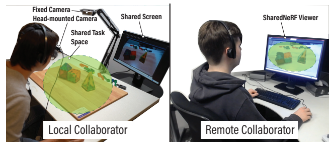
Figure 2: SHAREDNeRF local and remote setups. The local collaborator wears a head-mounted camera for real-time data collection and has a fixed camera on a desk for detecting movements in the task space (left). The remote collaborator uses the SHAREDNeRF viewer using a mouse and keyboard, navigating in the shared space (right).
