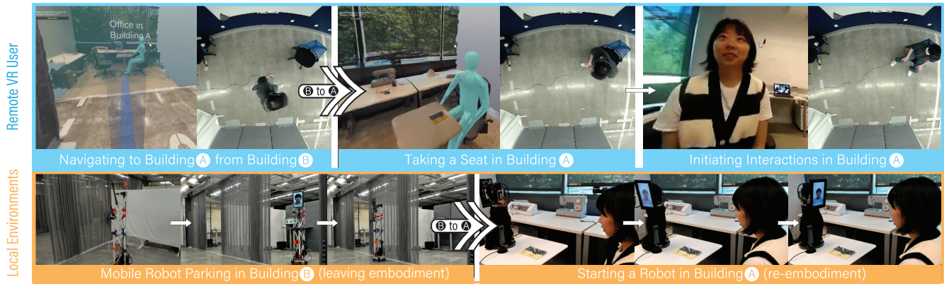
Figure 11: Demonstrations of switching between robotic proxies across multiple buildings. Using VRoxy, the VR user can navigate from the lab space in Building B to the office in Building A where the fixed robot is located to meet another collaborator. On the other side, the mobile robot in Building B starts parking to indicate the leave, and the stationary robot in Building A turns the body to face the collaborator to signify the re-embodiment.
