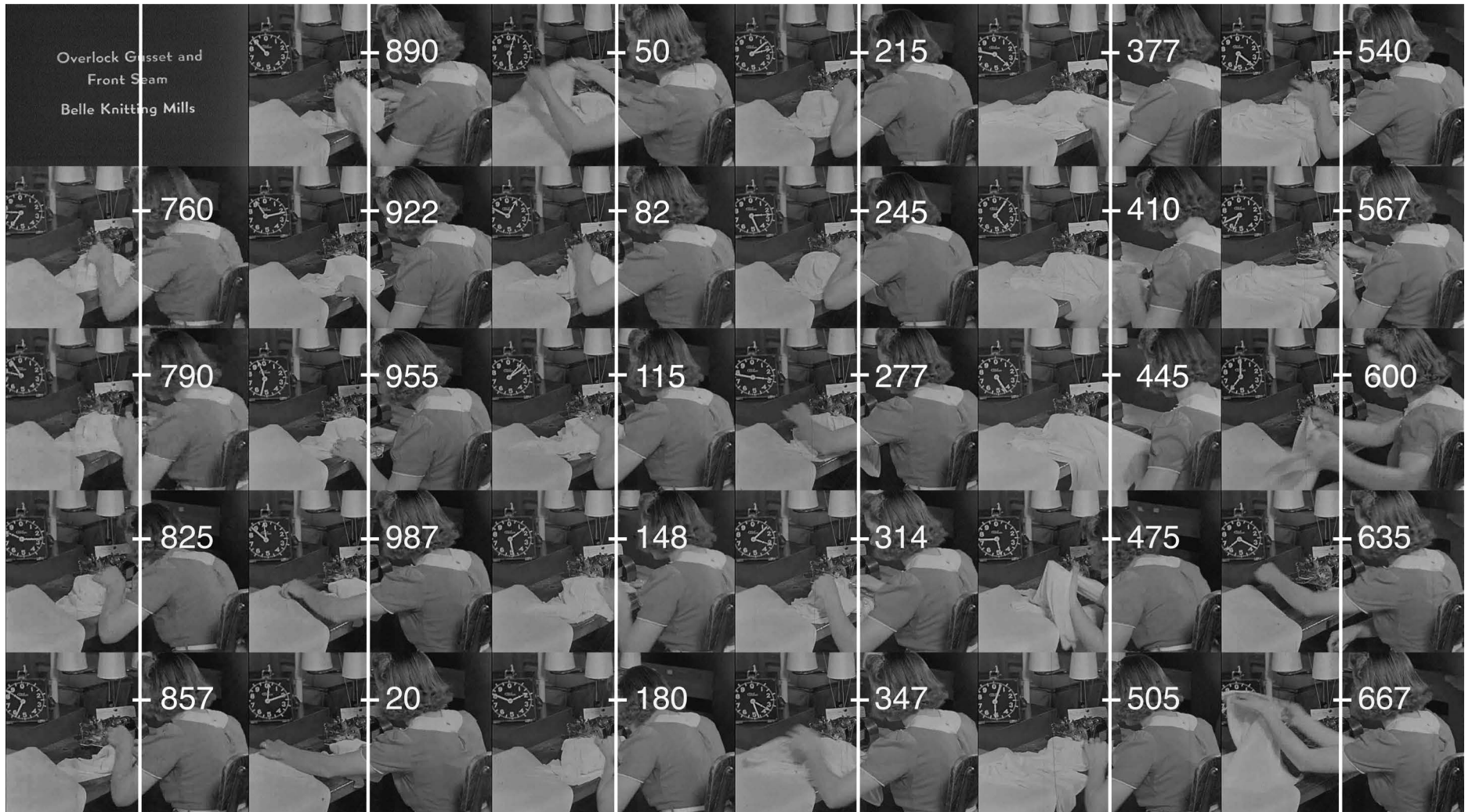
Archival film from Belle Knitting documenting an operator sewing an overlock gusset and front seam [29] with transcribed time (microchronometer reading) overlay.
